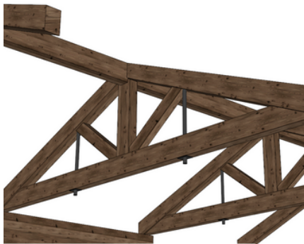
Fig. 3 - Small multiweb truss profile using metal rods.
